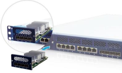
The PulM networking module marked with "A" must be installed into the slot with an "A" mark; so does the "B" module.
